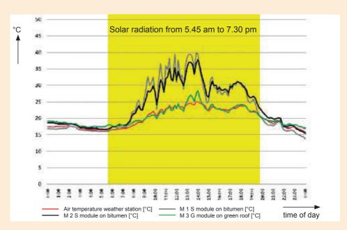
Graph: example of temperature graph recorded on 6 July 2009. The temperature of the modules on the bituminous panels (black and grey lines) rises to almost  $40^{\circ}$ C, while that of the module on the green roof (green line) does not go beyond a maximum of 27 °C and is, therefore, close to the ambient temperature (red line).
