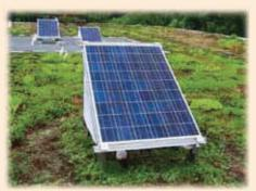
installed on "naked" bituminous panels being compared with one module installed on a green roof. In each case, attention was focused on the temperature at the underside
